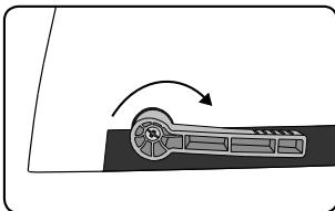
3. Ensure the comb-opening mechanism is closed.
