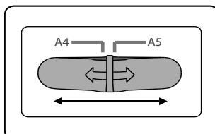
1. Select either A4 or A5 paper size and test punch scrap sheets. Select the correct comb diameter to suit the document (see chart).
