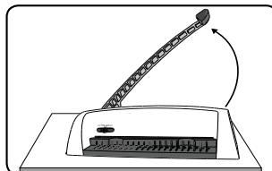
1. Ensure the machine is on a stable surface. Lift the punch handle to its upright position.
