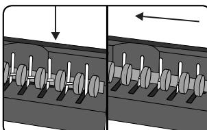
2. Place the binding comb into the opening mechanism and fully engage the opening plate by sliding the comb to the left.
